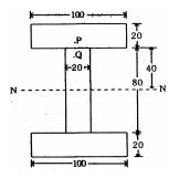
The shear stress at point P (very close to the bottom of the flange) is 12 MPa. The stress at point Q in the web (very close to the flange) is
